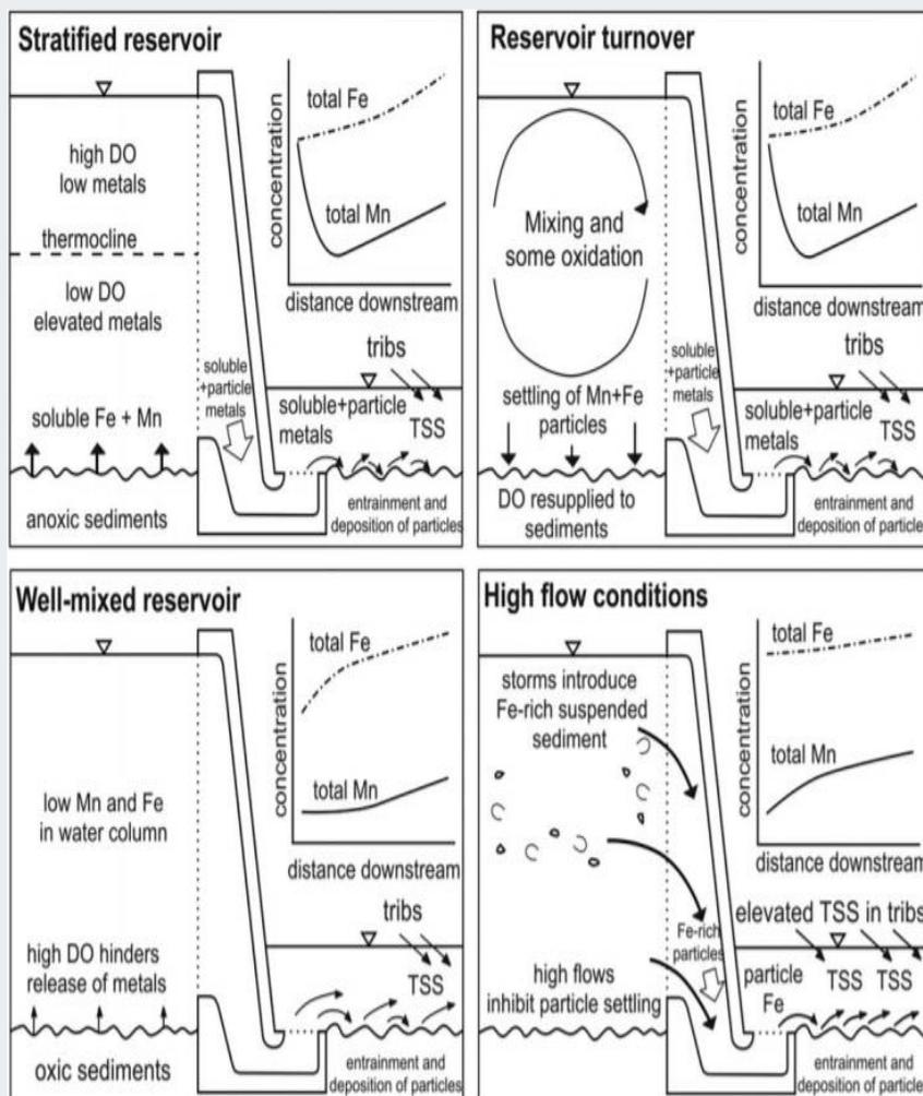
**Figure 2** - Metal cycles in a hydropower dam watershed in response to seasonal reservoir conditions and flow downgradient of the dam. DO = dissolved oxygen; FE = iron; MN = manganese; TSS = total suspended sediment (Image courtesy of Dr. Thomas Shahady)
